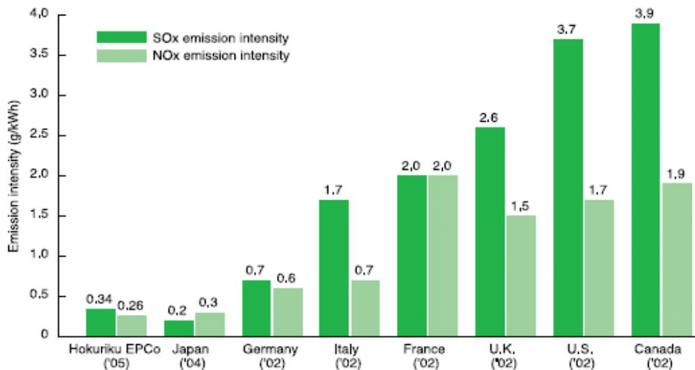
SOx and NOx emission intensities: SOx and NOx emissions per 1 kWh of electricity generated by a thermal power station.
