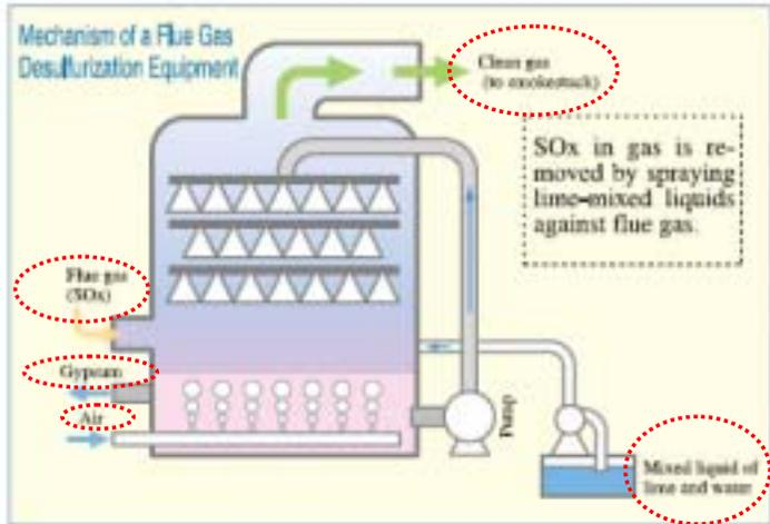
The gypsum generated from the desulfurizer as a by-product is recycled as cement material and gypsum board.
